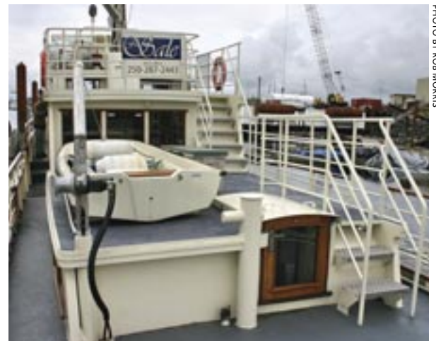
The aft companionway hatch hinges upward on air shocks and the mast pivots down on a hydraulic cylinder. The railings are painted stainless steel with teak caps. Owner John Dolmage, a long-time towboat, installed a tow-post and aft railings that can be removed because you never know when there might be an opportunity to do a tow job. Up on the bridge is a searchlight of the type originally installed on the seiner and manufactured by Magnet Electric, a still-operating Vancouver company (now Van-Mar Electric), which Capt. Bill Dolmage acquired after WWII.
